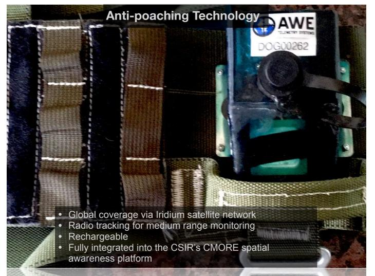
L-RAD and ANIRAD collars is automatically relayed to the AWE portal for online viewing or download. The base stations have satellite and GSM connectivity, making it easy to deploy a network.
